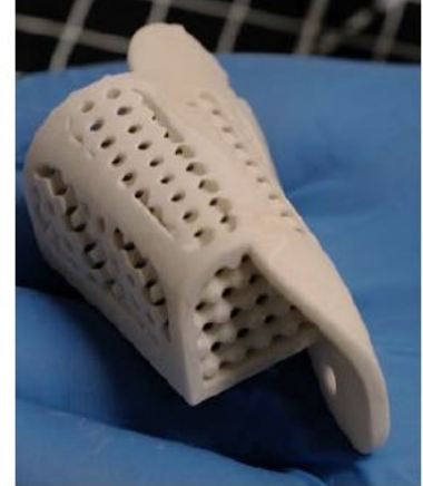
Fig 2: 3 D printed full ceramic mandible scaffold (6 cm)
